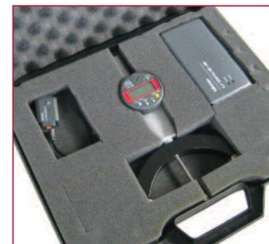
A specific wireless interface (optional) allows you to get and automatically send to the **CNC-C** the radius up to 25 m. long. This allows the creation and automatic editing of bending radius and any other kind of control.
