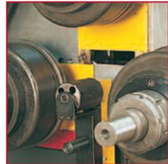
The machine performs all the operations necessary to complete desired shape until the bent profile comes out from the bending machine.
